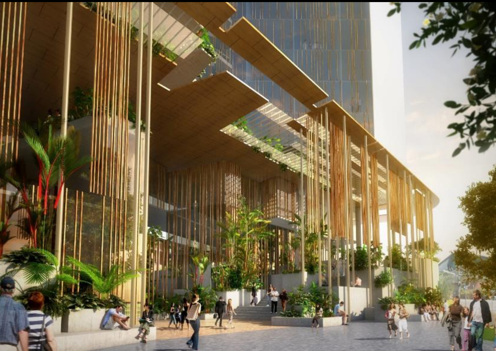
Deep shaded occupied edges for west and east facing buildings
