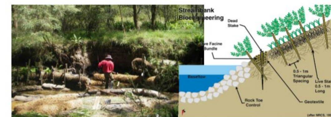
Geotextile revetment of Yosemite Creek, Blue Mountains. Photo: Geoffrey Smith. Geotextile fabrics planted out with vegetation to stabilise a stream bank. Taken from Iowa State University Forestry Department. http://www.buffer.forestry.iastate.edu/Assets/streambioeng.gif
