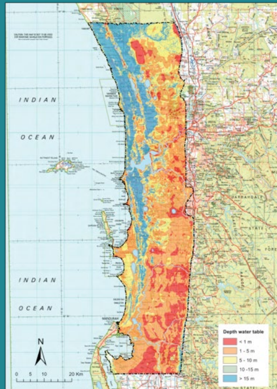
Figure 1. Depth to groundwater across the Perth coastal plain ranges from greater than 15 metres to less than one metre.
