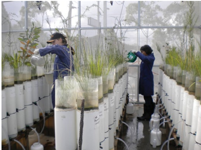
Figure 1. Dosing laboratory-scale biofilter columns using semi-synthetic stormwater (© Monash University).
