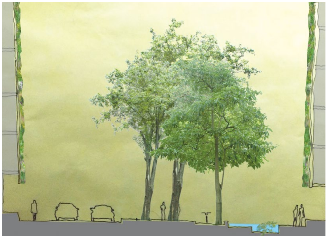
Figure 16. A green canyon – comprising green walls and trees – can be up to 6 °C cooler than surrounding areas during extreme heat conditions
