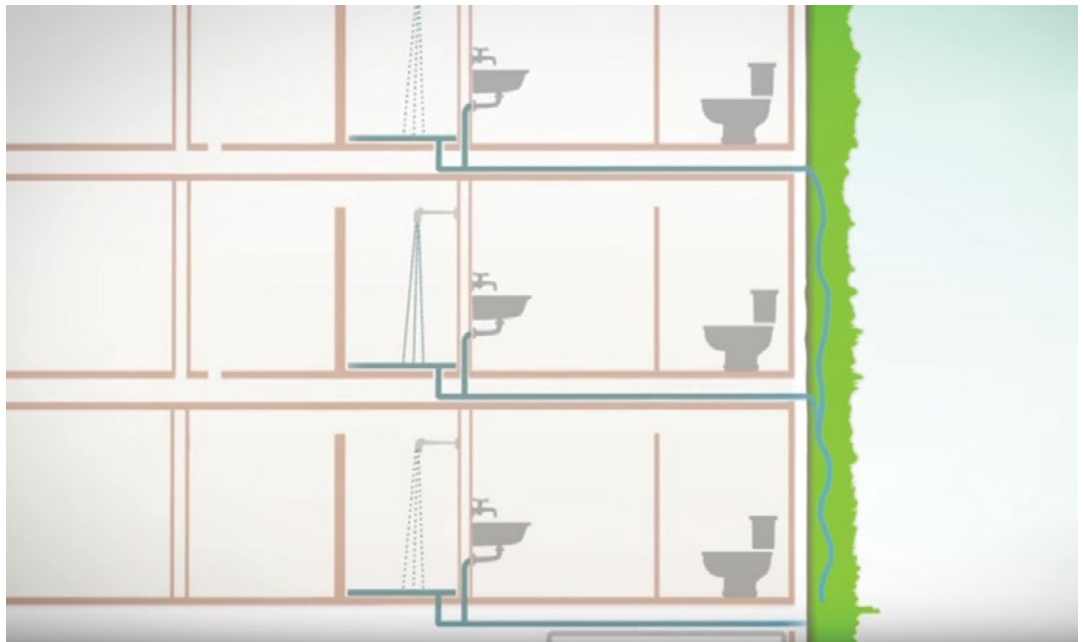
Figure 15. Greywater reuse using green walls. The green wall is maintained by the regular flows of greywater while also acting as a biofilter to remove chemicals and pathogens, allowing excess greywater to be used as a resource.
