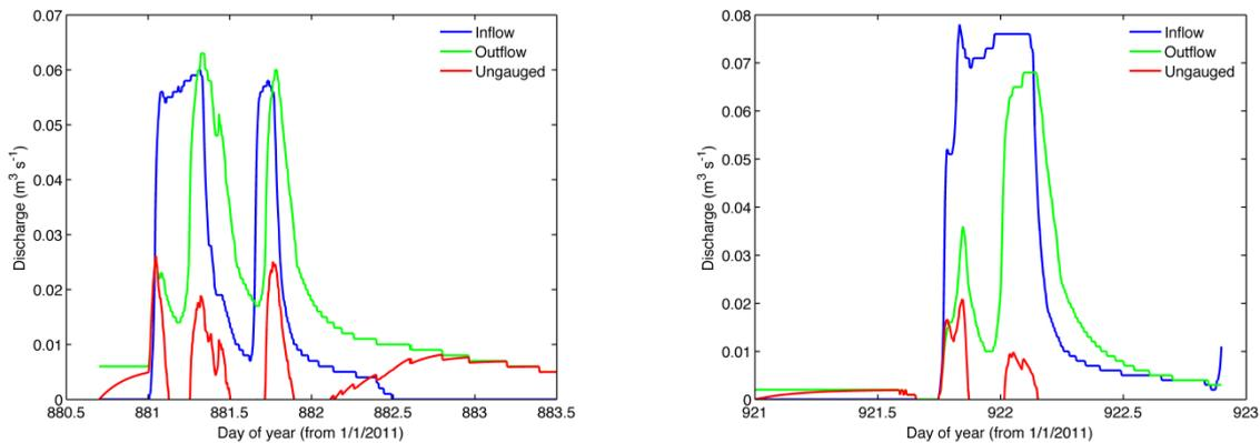
**Figure 6. Resulting hydrographs from large rainfall event under dry antecedent conditions on 29/05/2013 (left) and 09/07/2013 (right). Ungaugged hydrograph (red line) was obtained as the difference between outflow hydrograph and the routing of the inflow hydrograph using a linear storage routing technique.**
