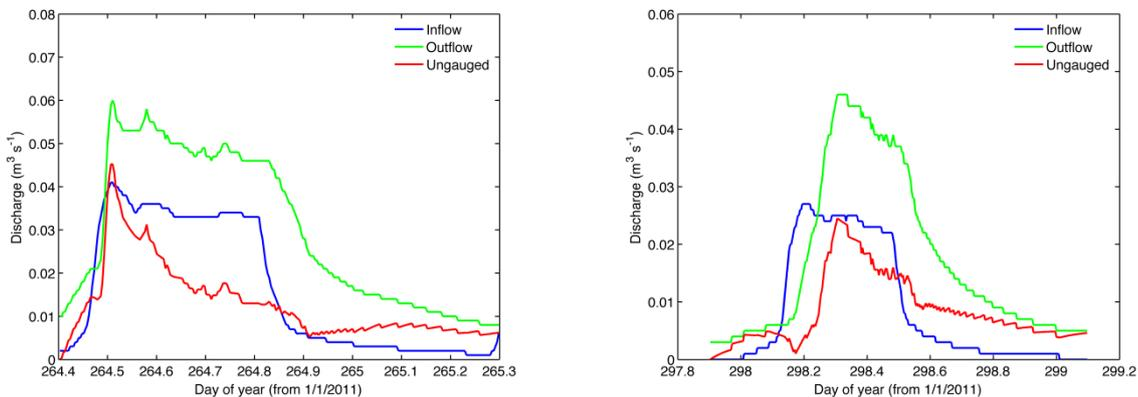
**Figure 8. Resulting hydrographs from high intensity rainfall events on 21/09/2011 (left) and 24/10/2011 (right). Ungaugged hydrograph (red line) was obtained as the difference between outflow hydrograph and the routing of the inflow hydrograph using a linear storage routing technique.**
