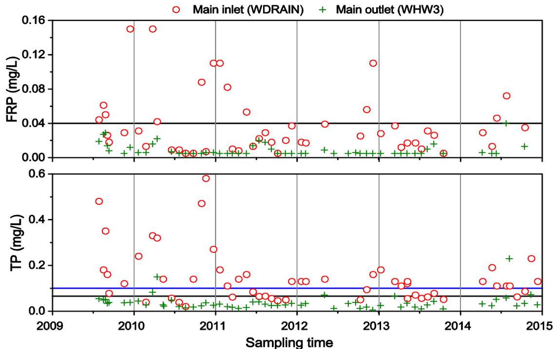
Figure 18. Variation of concentrations of phosphorus species in water at main inlet (WDRAIN) and main outlet (WHW3) of Wharf Street Constructed Wetland. Solid horizontal dark lines show the ANZECC guidelines and horizontal blue lines show Healthy Rivers target values.
