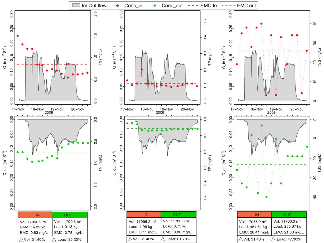
Figure 28. Flow and nutrient dynamics at the main inlet and outlet from 17 to 20 November 2009.
