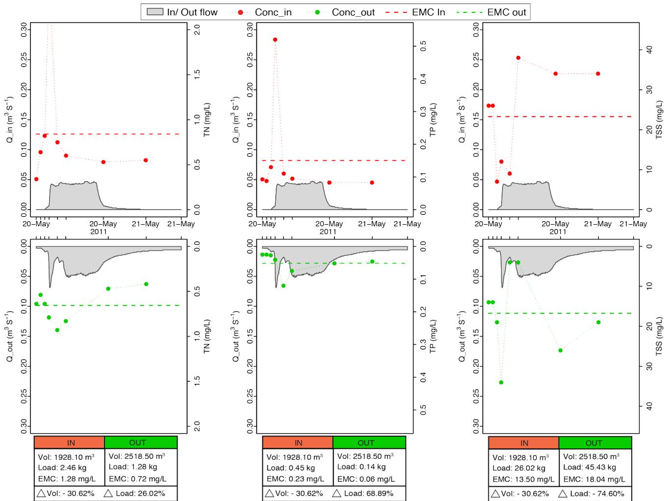
**Figure 30. Flow and nutrient dynamics at the main inlet and outlet from 20 to 21 May 2010.**
