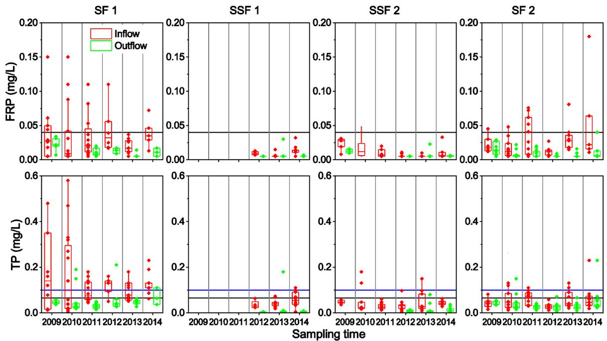
Figure 17. Annual distribution of phosphorus species in water at different components of Wharf Street Constructed Wetland. Solid horizontal lines within individual boxes indicates the median value of the data set and lower and upper parts of the boxes indicate 75 and 25 percentile of data. Solid horizontal dark lines show the ANZECC guidelines and horizontal blue lines show Healthy Rivers target values. Laterite-based SSF 1 and SSF 2 started operation in October 2012.
