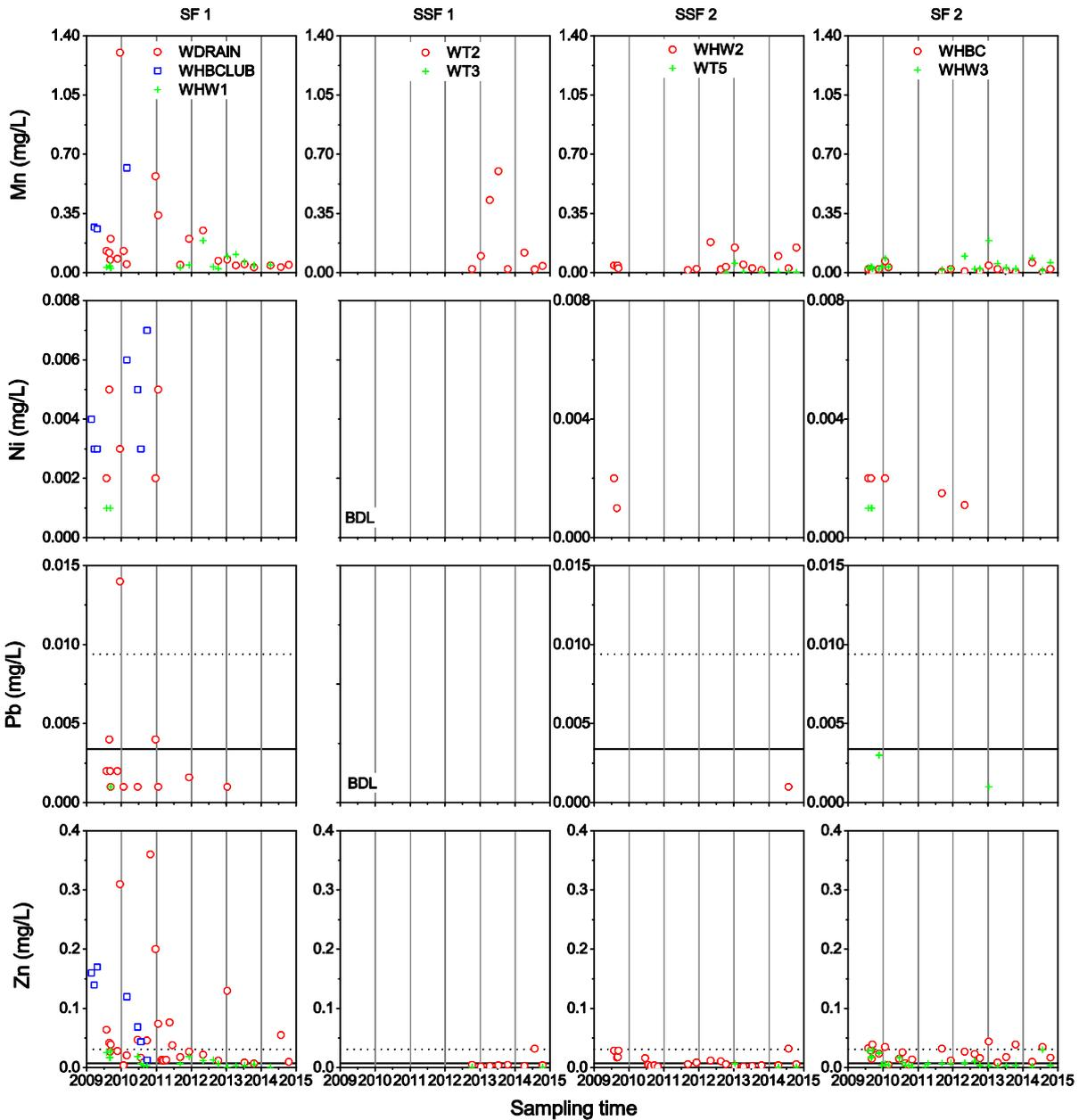
Figure 20. Spatial and temporal variation of metal concentrations in water at different sampling points throughout the components of Wharf Street Constructed Wetland. Horizontal dashed and solid lines show the ANZECC 80% and 95% trigger values respectively. BDL denotes below detectable limit. Laterite-based SSF 1 and SSF 2 started operation in October 2012.
