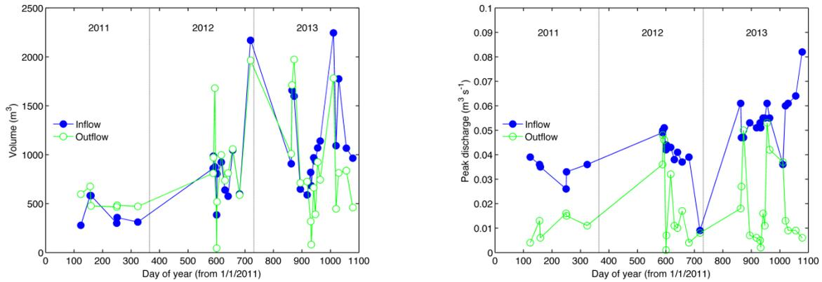
**Figure 2. Temporal variability of pumping event characteristics over the study period: total water volume (left) and peak discharge (right) for each individual event.**
