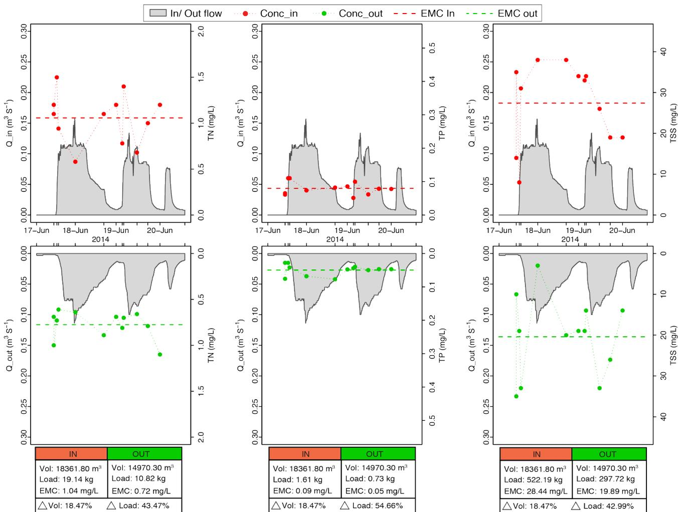
**Figure 33. Flow and nutrient dynamics at the main inlet and outlet from 17 to 20 June 2014.**
