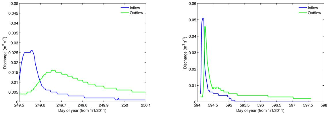
**Figure 3. Pumping event hydrographs under wet antecedent condition, on 06/09/2011(left) and 16/08/2012 (right).**
