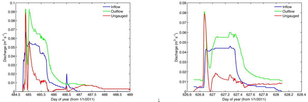
**Figure 5. Resulting hydrographs from large rainfall events under wet antecedent conditions on 28/04/2012 (left) and 17/09/2012 (right). Ungaugged hydrograph (red line) was obtained as the difference between outflow hydrograph and the routing of the inflow hydrograph using a linear storage routing technique.**
