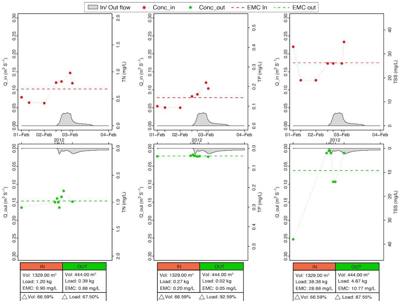
**Figure 31. Flow and nutrient dynamics at main inlet and outlet from 1 to 4 February 2012.**
