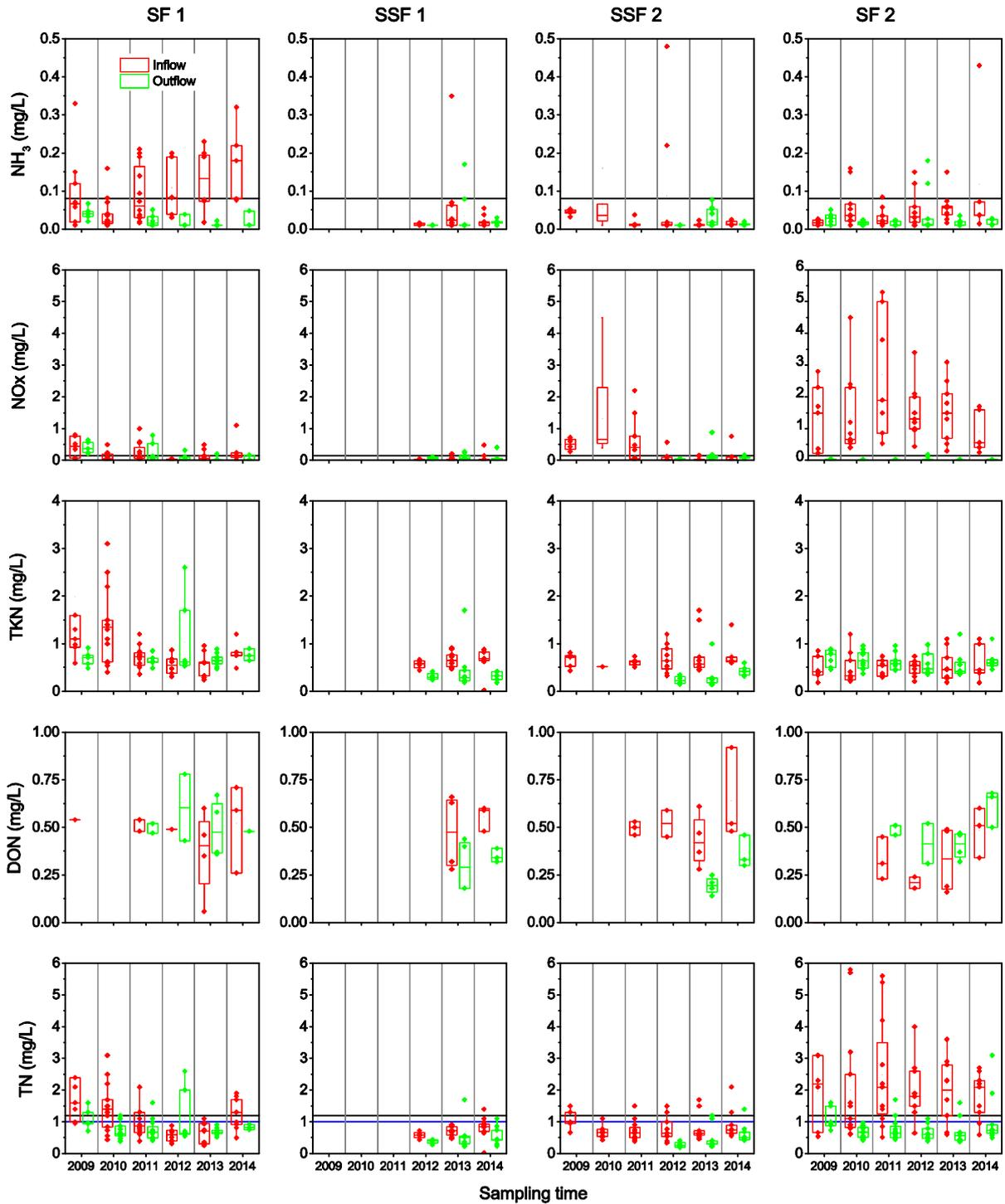
Figure 14. Annual distribution of nitrogen species in water within different components of the Wharf Street Constructed Wetland. Solid horizontal lines within individual boxes indicate the median value of the data set and lower and upper parts of the boxes indicate 75 and 25 percentile of data. Solid horizontal dark lines show the ANZECC guidelines and horizontal blue lines show Healthy Rivers target values. Laterite-based SSF 1 and SSF 2 started operation in October 2012.
