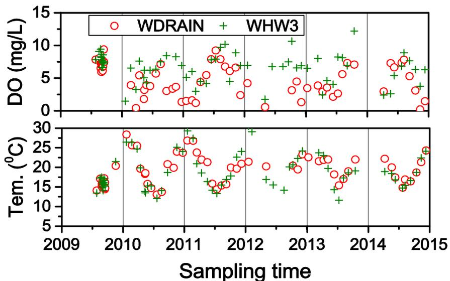
Figure 12. Variation of DO concentrations and water temperature at main inlet (WDRAIN) and main outlet (WHW3) of Wharf Street Constructed Wetland from 2009 to 2014.
