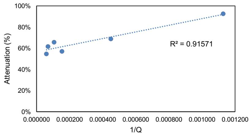
Figure 35. TP attenuation based on storm magnitude (1/Q, relative units) during six storm events.
