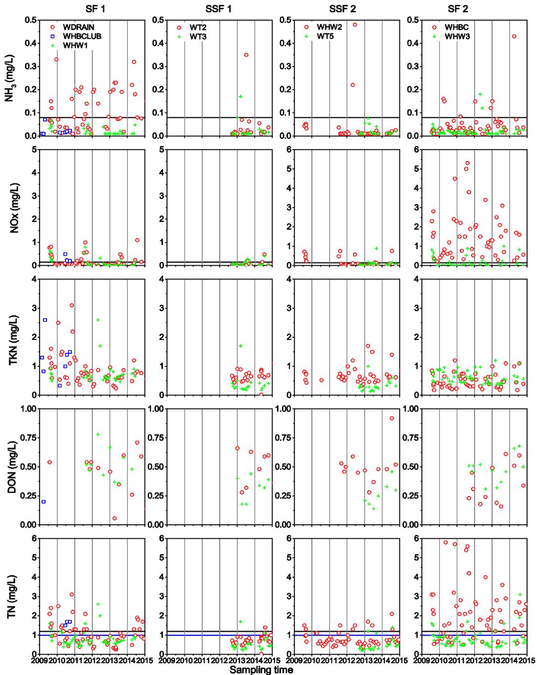
Figure 13. Spatial and temporal variation of concentrations of nitrogen species in water at different sampling points throughout the components of the Wharf Street Constructed Wetland. Solid horizontal dark lines show the ANZECC guidelines and horizontal blue lines show Healthy Rivers target values. Laterite-based SSF 1 and SSF 2 started operation in October 2012.
