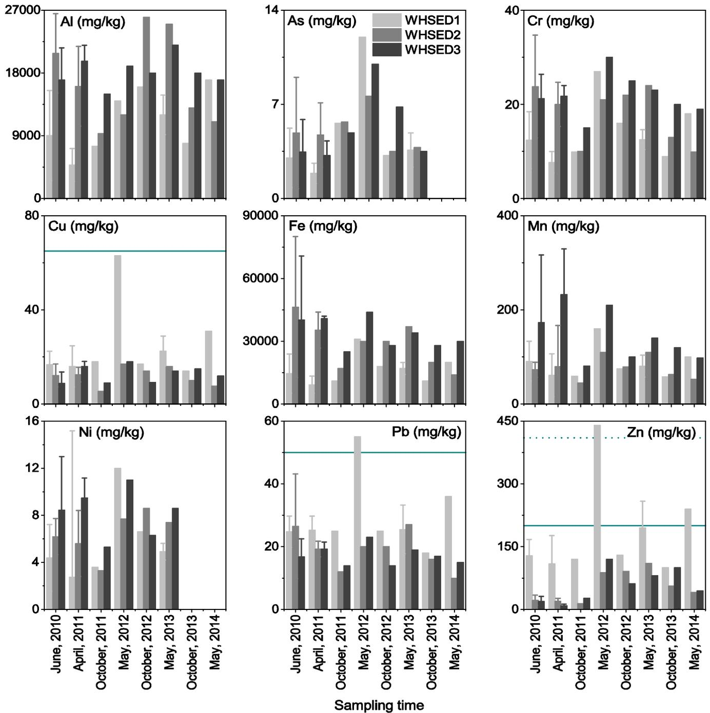
Figure 40. Spatial and temporal variation of metal content in the sediment of the Wharf Street Constructed Wetland. Horizontal solid and dashed dark lines in each plot represent the ISQG-low (trigger value) and ISHG-high (trigger value), respectively.
