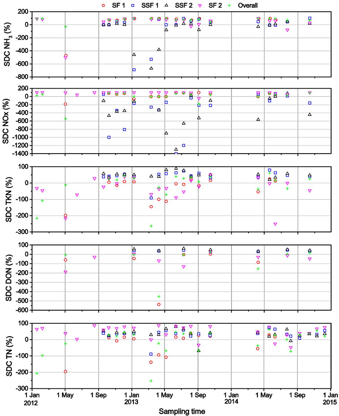
Figure 23. Attenuation (%) of nitrogen species at different components of the Wharf Street Constructed Wetland from 2012 to 2014. Positive and negative SDC indicate nutrient reduction and increase, respectively. See Table 1 for nomenclature of the different components.
