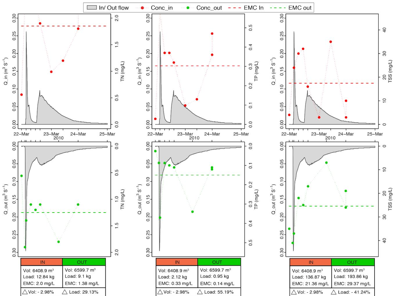
Figure 29. Flow and nutrient dynamics at the main inlet and outlet from 23 to 25 March 2010.
