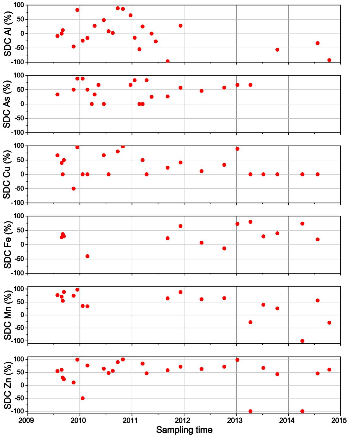
Figure 37. Metal attenuation (%) in the Wharf Street Constructed Wetland from 2009 to 2014. Positive SDC indicates metal reduction while negative indicates metal increases.
