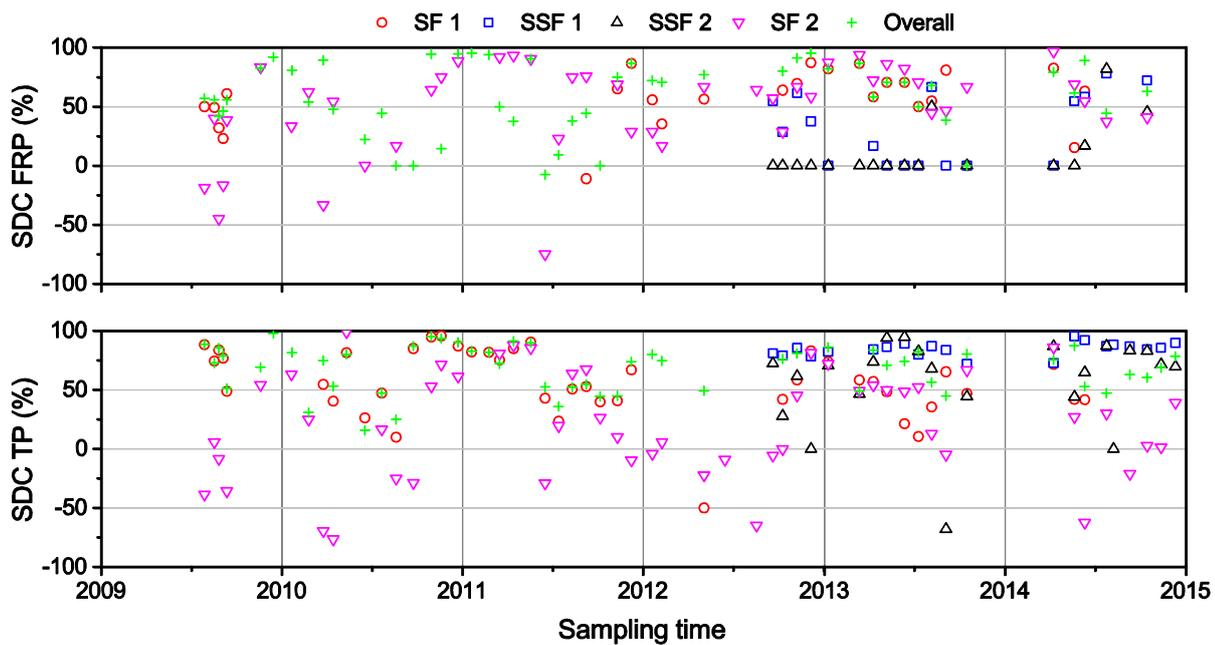
Figure 25. Attenuation (%) of phosphorus species at different components of the Wharf Street Constructed Wetland from 2009 to 2014. Positive and negative SDC indicate nutrient reduction and increase, respectively. See Table 1 for nomenclature of different components.
