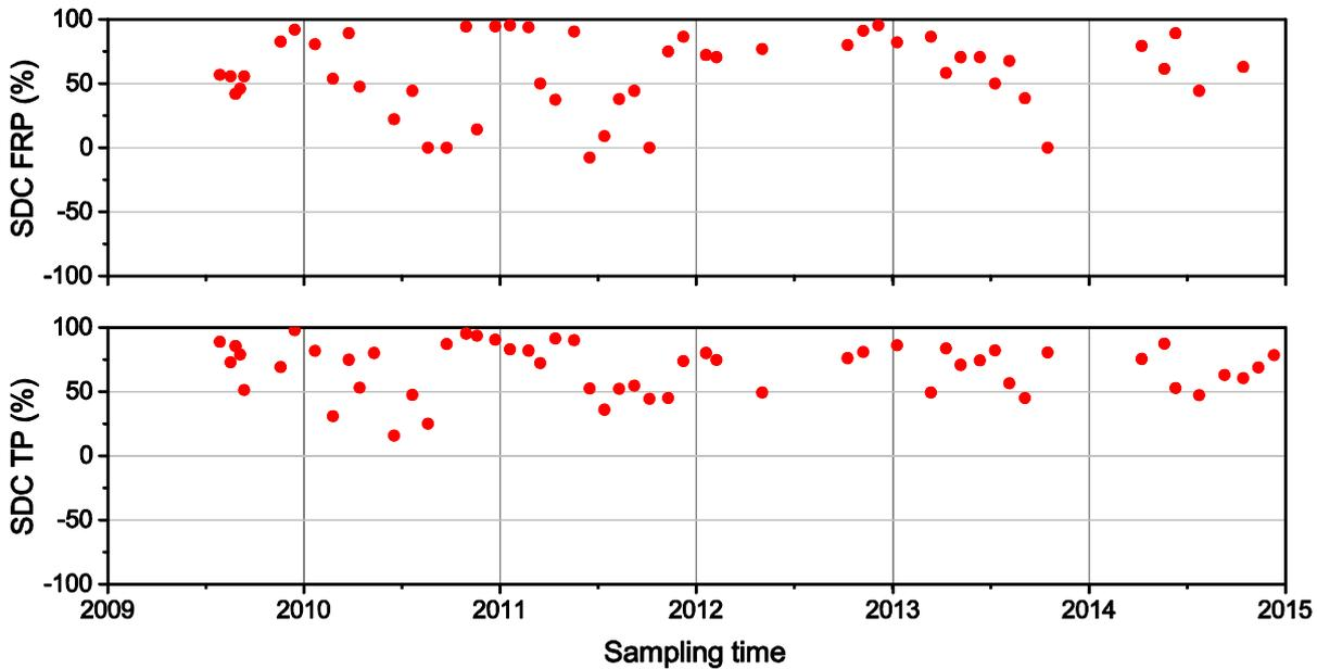
Figure 27. Overall attenuation (%) of phosphorus species by Wharf Street Constructed Wetland from 2009 to 2014. Baseflow nutrient data from the main inlet and main outlet were considered. Positive and negative SDC indicate nutrient reduction and increase, respectively.
