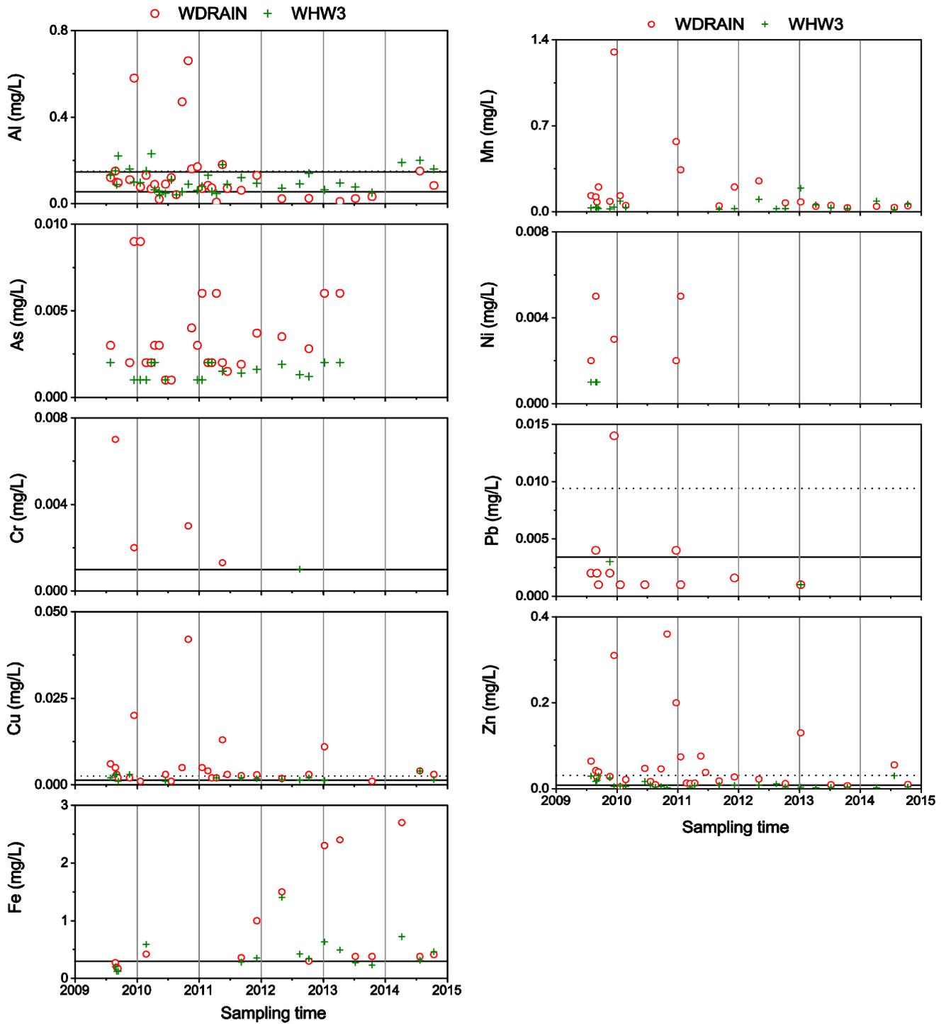
Figure 21. Metal concentrations in water at the main inlet and main outlet of Wharf Street Constructed Wetland. Horizontal dashed and solid lines show the ANZECC 80% and 95% trigger values respectively.
