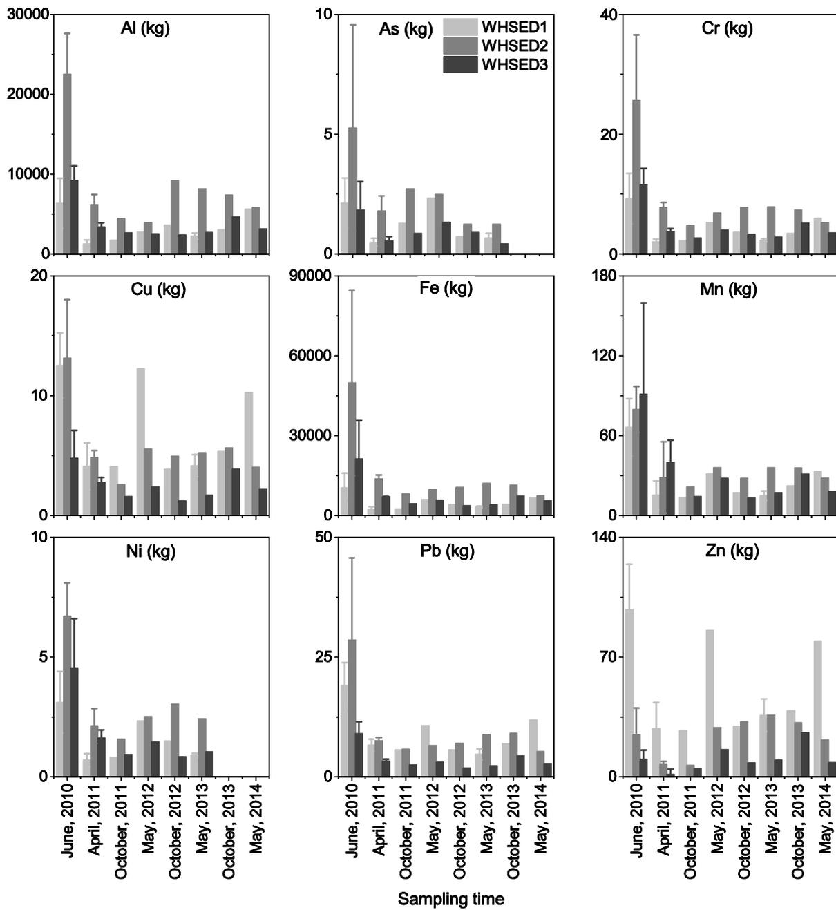
Figure 41. Spatial and temporal variability of mass of metals in the sediment at Wharf Street Constructed Wetland. Vertical line and bar indicates the standard deviation.
