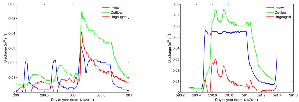
Figure 4. Resulting hydrographs from a combined pump-rainfall events on 26/10/2011 (left) and 11/08/2012 (right). Ungauged hydrograph (red line) was obtained as the difference between outflow hydrograph and the routing of the inflow hydrograph using a linear storage routing technique.
