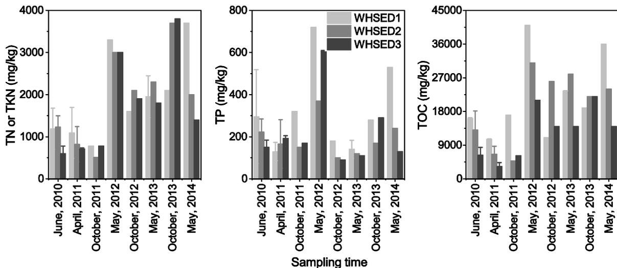
Figure 38. Spatial and temporal variation of TKN or TN, TP and TOC concentrations in the sediment at the Wharf Street Constructed Wetland (mean and standard deviations).
