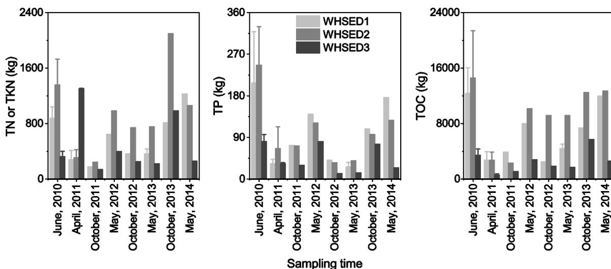
Figure 39. Spatial and temporal variability of nutrient mass in the sediments at the Wharf Street Constructed Wetland (average and standard deviations).
