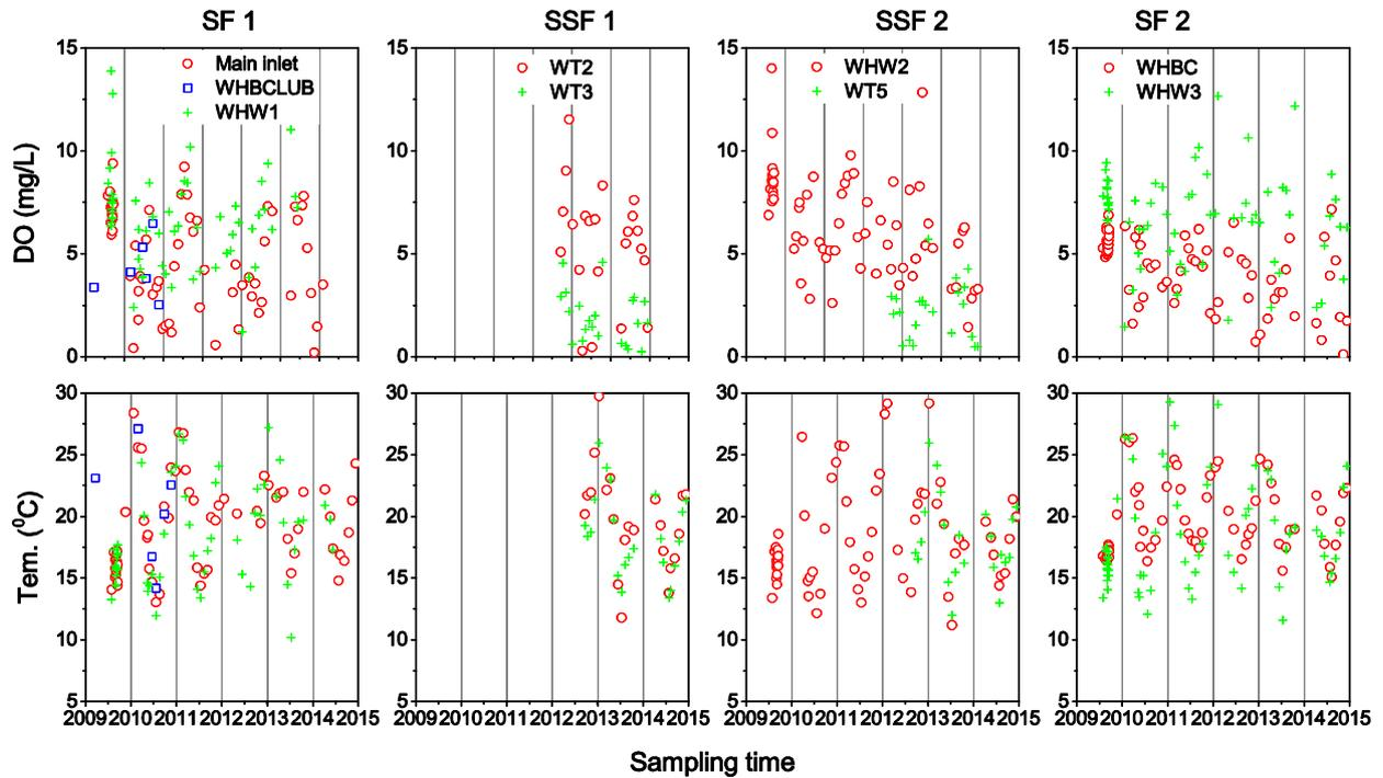
Figure 11. Spatial and temporal variation of dissolved oxygen (DO) concentration and water temperature (Tem) at different sampling points throughout the components of Wharf Street Constructed Wetland. Laterite-based SSF 1 and SSF 2 started operation in October 2012.
