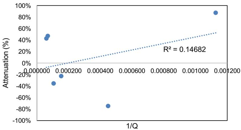
Figure 36. TSS attenuation based on storm magnitude (1/Q, relative units) during six storm events.
