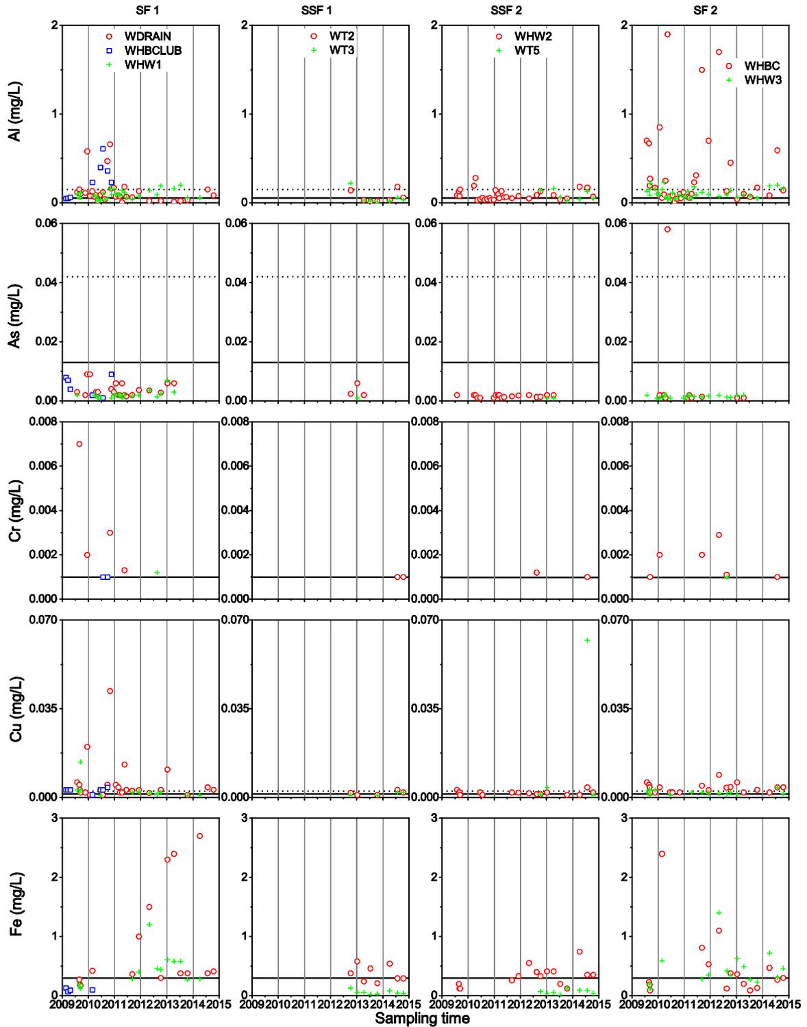
Figure 19. Spatial and temporal variation of metal content in water at different sampling points throughout the compartments of Wharf Street Constructed Wetland. Horizontal dashed and solid lines show the ANZECC 80% and 95% trigger values respectively. BDL denotes below detectable limit. Laterite-based SSF 1 and SSF 2 started operation in October 2012.
