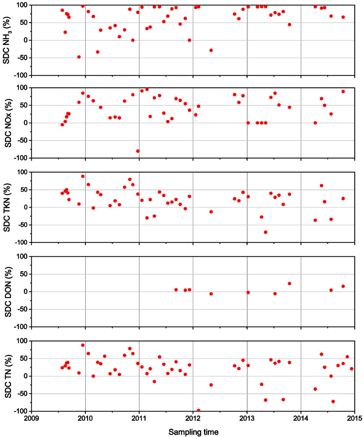
Figure 24. Overall attenuation (%) of nitrogen species by the Wharf Street Constructed Wetland from 2009 to 2014. Baseflow nutrient data from the main inlet and main outlet were considered. Positive and negative SDC indicate nutrient reduction and increase, respectively.
