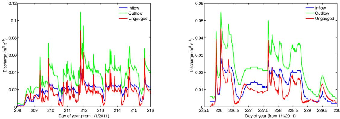
**Figure 7. Resulting hydrographs from frequent rainfall events under wet antecedent conditions on 27/07/2011 (left) and 13/08/2011 (right). Ungaugged hydrograph (red line) was obtained as the difference between outflow hydrograph and the routing of the inflow hydrograph using a linear storage routing technique.**
