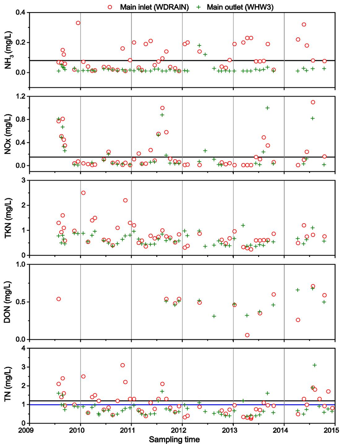
Figure 15. Variation of concentrations of nitrogen species in water at main inlet (WDRAIN)m and main outlet (WHW3) of Wharf Street Constructed Wetland. Solid horizontal dark lines show the ANZECC guidelines and horizontal blue lines show Healthy Rivers target values.
