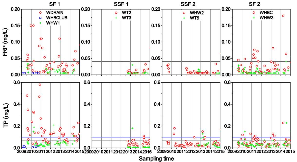
Figure 16. Spatial and temporal variation of concentrations of phosphorus species in water at different sampling points throughout the components of Wharf Street Constructed Wetland. Solid horizontal dark lines show the ANZECC guidelines and horizontal blue lines show Health Rivers target values. Laterite-based SSF 1 and SSF 2 started operation in October 2012.
