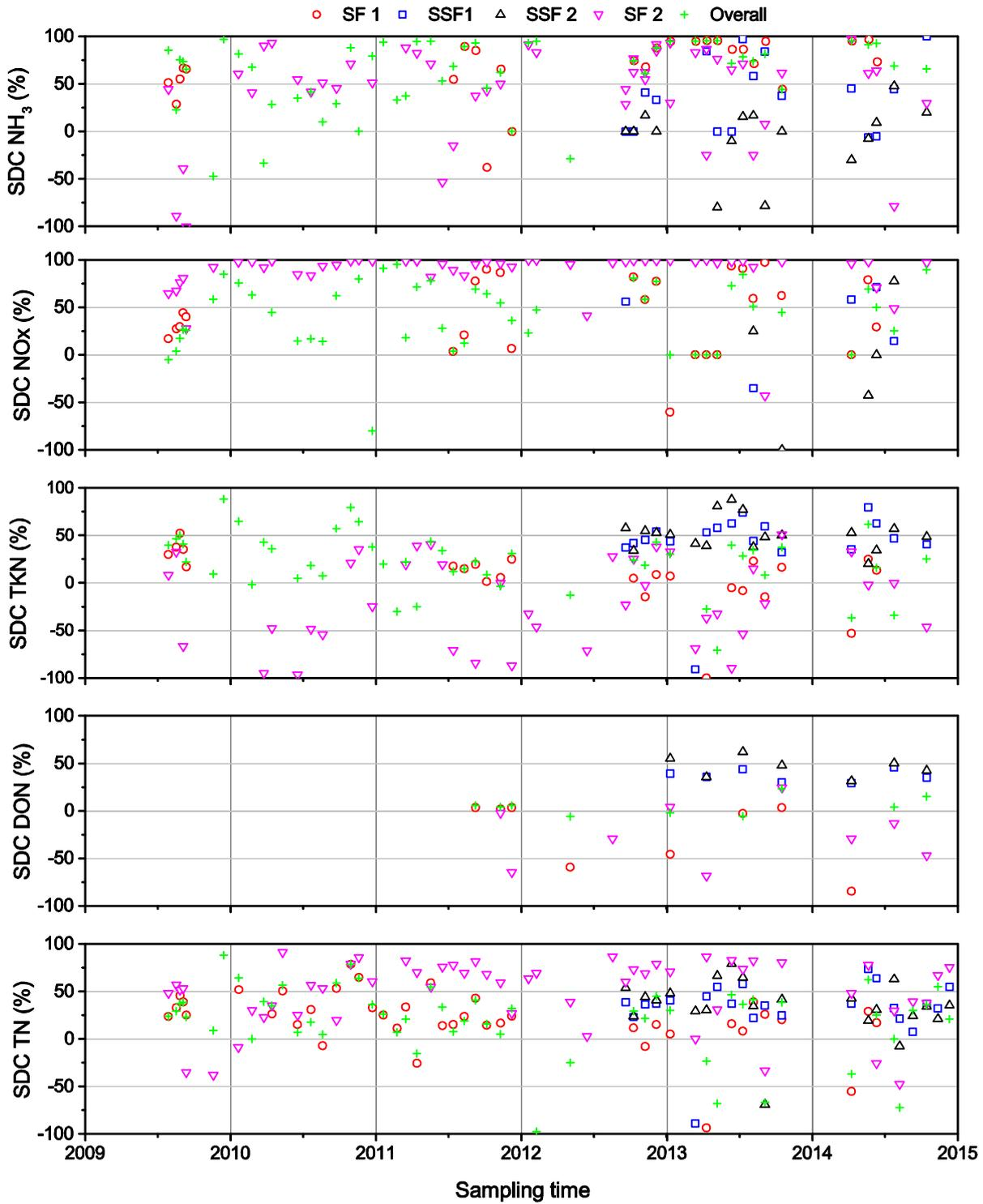
Figure 22. Attenuation (%) of nitrogen species at different components of the Wharf Street Constructed Wetland from 2009 to 2014. Positive and negative SDC indicate nutrient reduction and increase, respectively. See Table 1 for nomenclature of the different components.
