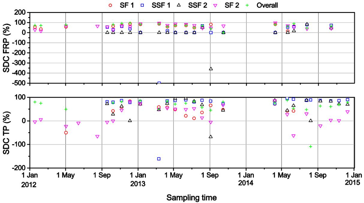
Figure 26. Attenuation (%) of phosphorus species at different components of the Wharf Street Constructed Wetland from 2012 to 2014. Positive and negative SDC indicate nutrient reduction and increase, respectively. See Table 1 for nomenclature of different compartments.
