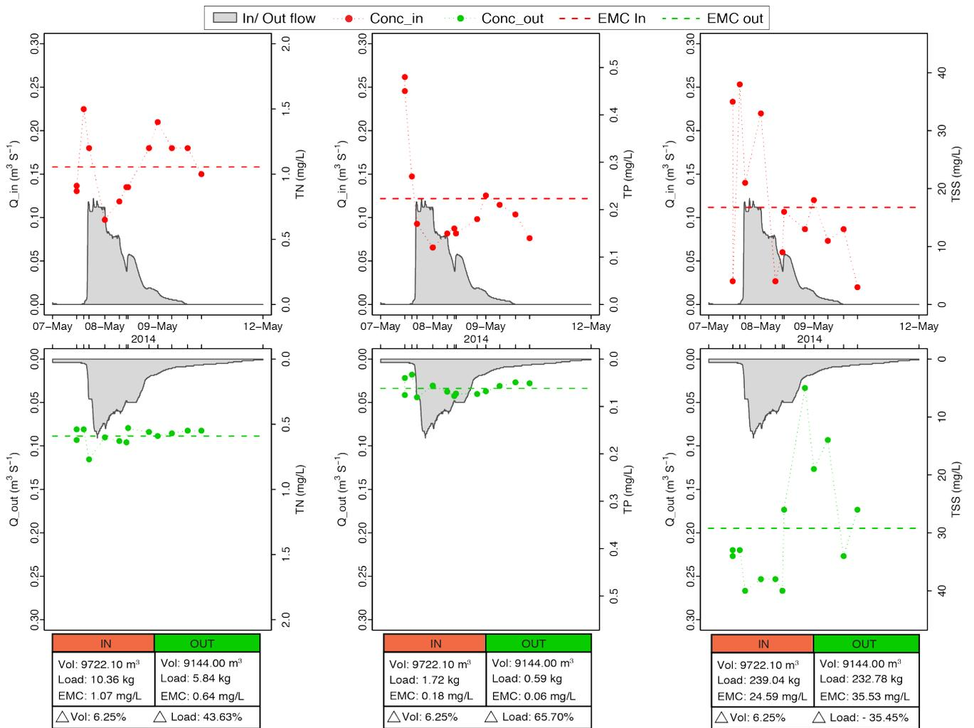
Figure 32. Flow and nutrient dynamics at the main inlet and outlet from 7 to 12 May 2014.
