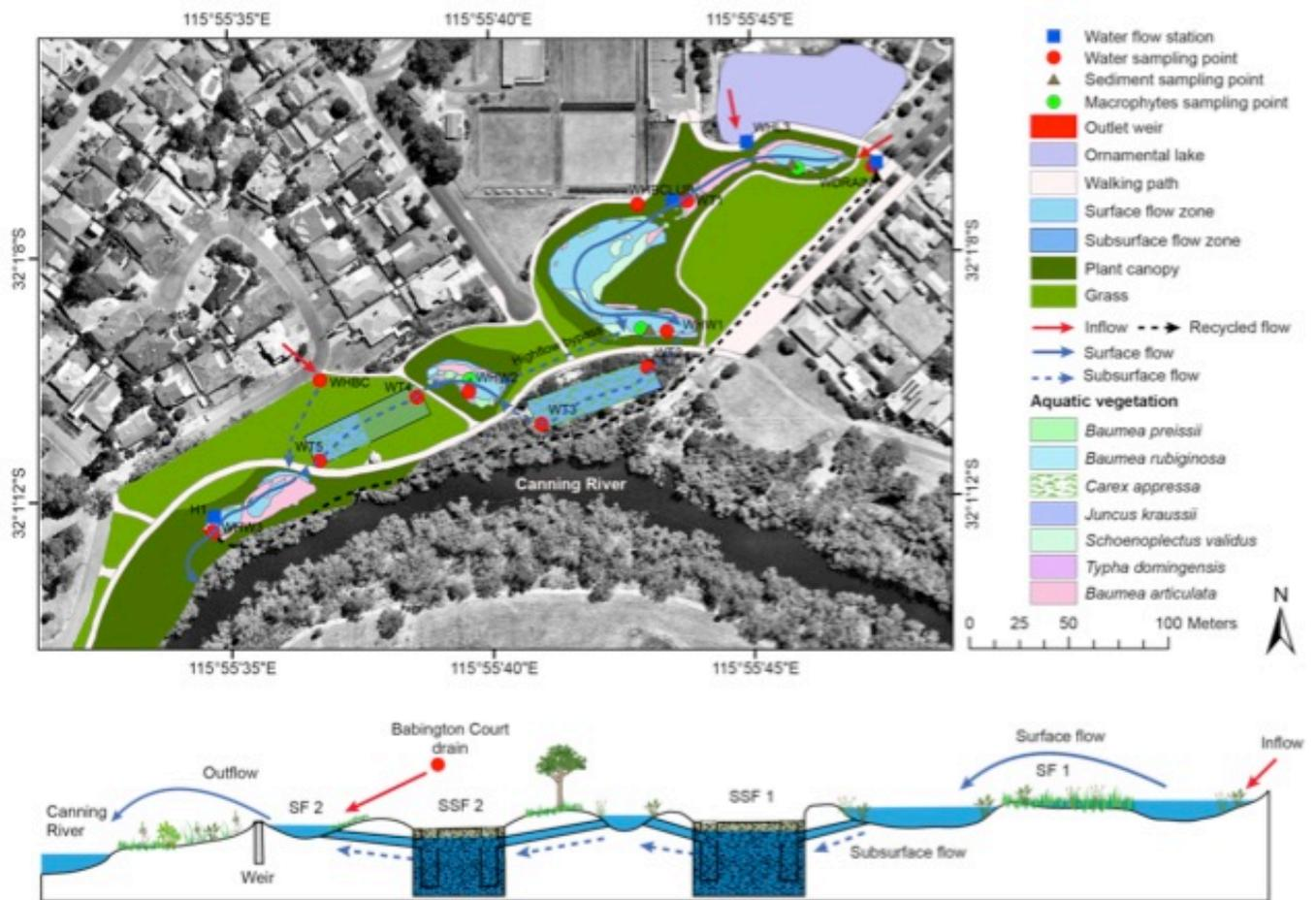
Figure 1. (Top panel) Map of Wharf Street Constructed Wetland indicating different sampling points of surface water, flow, sediment and macrophytes. (Bottom panel) Cross-section of flow path of the system through multistage surface flow and laterite-based subsurface flow components. Additional pipes allow sub-surface systems to be bypassed under high flow conditions and half of SSF2 is covered by grass.
