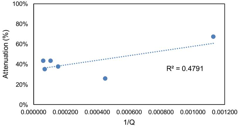
Figure 34. TN attenuation based on storm magnitude (1/Q, relative units) during six storm events.
