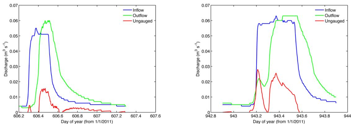
Figure 10. Resulting hydrographs from single-isolated rainfall event under wet antecedent condition: Events on 28/08/2012 (left) and 30/07/2013 (right). Ungauged hydrograph (red line) was obtained as the difference between outflow hydrograph and the routing of the inflow hydrograph using a linear storage routing technique.
