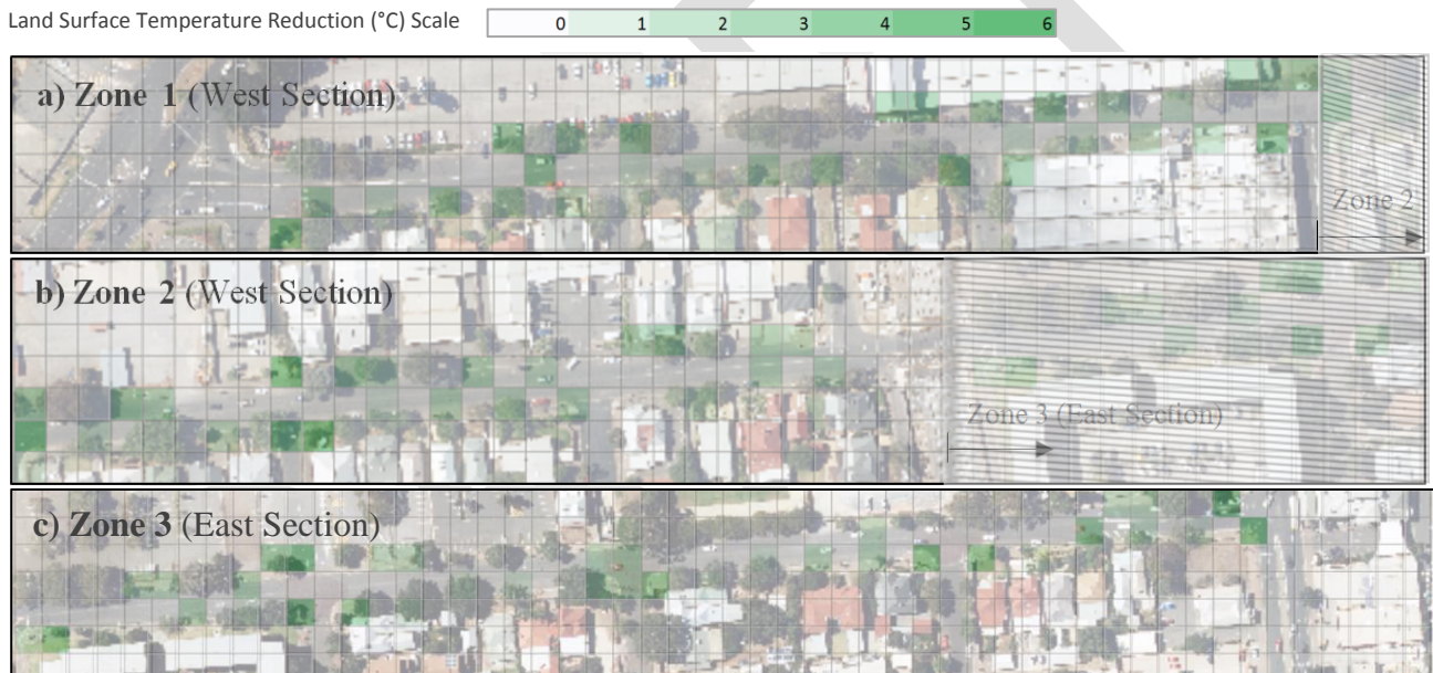
Figure 8 Land Surface Temperature reduction along the Leader Street (following full establishment of tree canopy)
