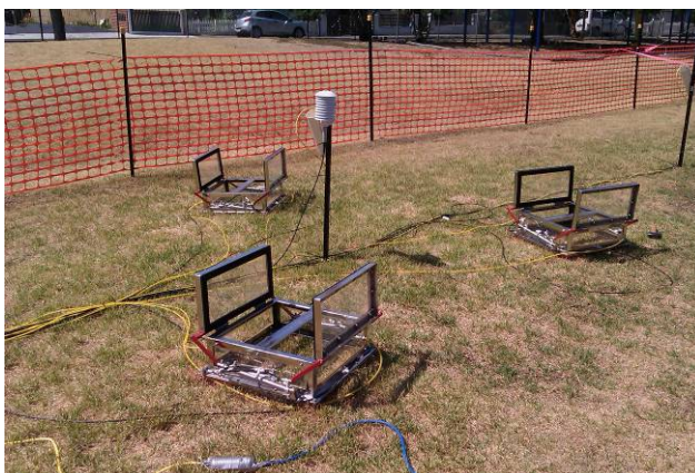
The location of the oval at Footscray P.S. and surrounding iButton sensors (upper-left), chambers for measuring evapotranspiration from the irrigation event (lower-left), and the masts to monitor downwind cooling effects (upper-right)
