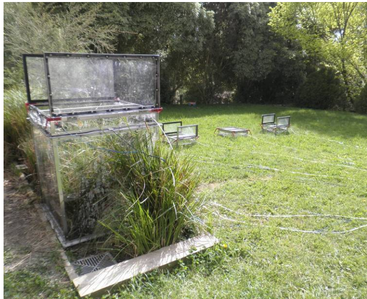
The evapotranspiration chambers on a transect starting next to the raingarden
