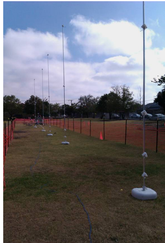
The location of the oval at Footscray P.S. and surrounding iButton sensors (upper-left), chambers for measuring evapotranspiration from the irrigation event (lower-left), and the masts to monitor downwind cooling effects (upper-right)
