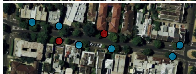
Bourke St (upper) in the Melbourne CBD, Gipps St (middle-treed) and George St (lower – non-treed) in East Melbourne and location of micro-climate monitoring stations in the open (red) and under the shaded by the tree canopy (blue)
