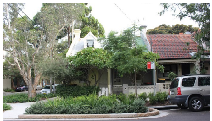
Design of a raingarden should reflect its context, including land use, predominant style of architecture, and plant selection in existing streetscape. A suitable design for a raingarden in one context might not be suitable in another. Photos: M. Dobbie
