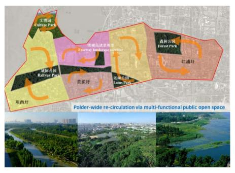
The multi-functional corridor integrates blue, green and grey infrastructure and form an iconic and integral part of urban ecology and at same time provide important passage for safe conveyance of floods. These corridors are created as a result of coordinated planning and implementation between various stakeholders.
