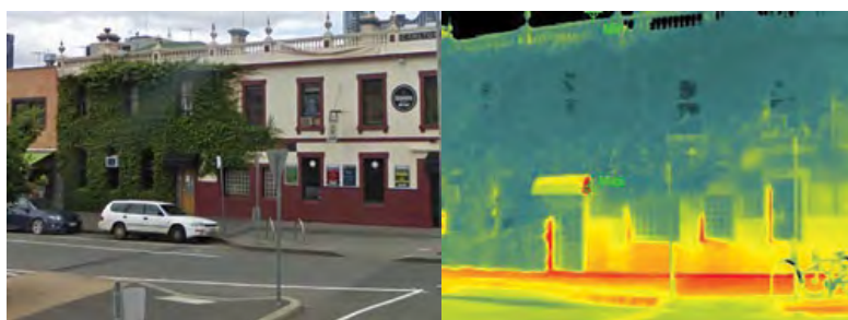
Figure 15 The cooling benefits of a green building facade on a 27°C day (Source: Coutts et al. 2014).
