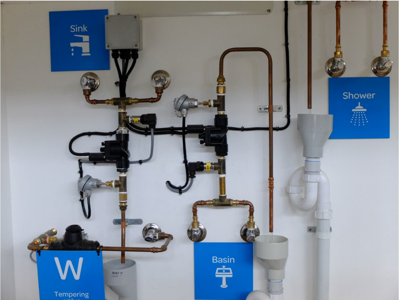
Trialling of rainwater to hot water connections at Holmesglen Tafe
