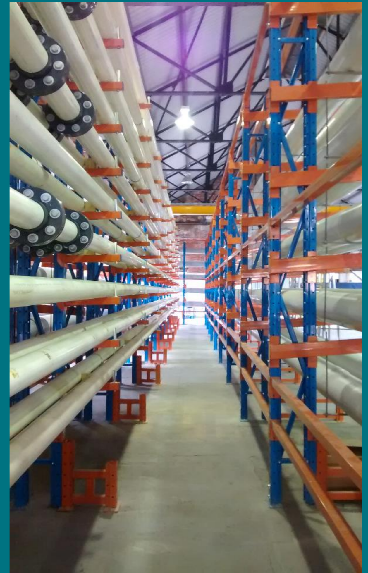
Pictured Above: The Innovation Centre Sewer Pilot allowed for this research to be carried out using two parallel 300 meter long pressure main pipes. With this, we were able to control critical variables while still mirroring real world conditions .
