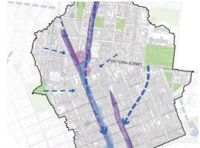
→ A map of the Elizabeth Street Catchment showing priority flood risk areas and flow directions
