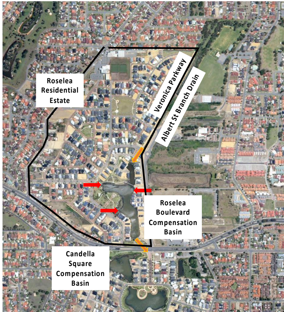
Figure 2. Albert St Branch Drain inflows and outflows (orange), and road runoff inflows (red) into the Roselea Blvd Compensation Basin (Nearmap, December 2009).
