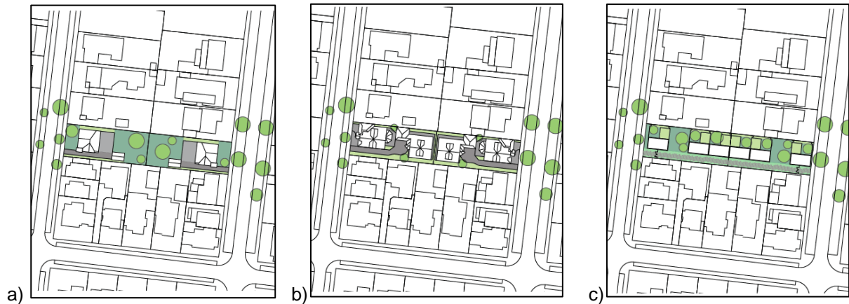
Figure 3: Three scenarios for houses on a typical middle suburban 2-lot site: a) Typical Existing - 2 single-storey detached houses; b) Business-as-usual (BAU) - 4 single-storey detached houses; c) Water sensitive (WS) - 6 two-storey integrated dwellings. (London et al., 2019)
