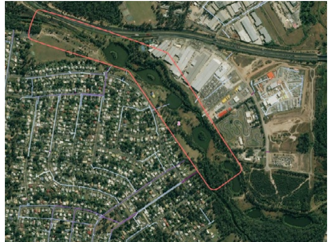
Figure 5. Aerial of JJ Smith Park Lakes (stormwater pipe network shown in blue-purple lines)
