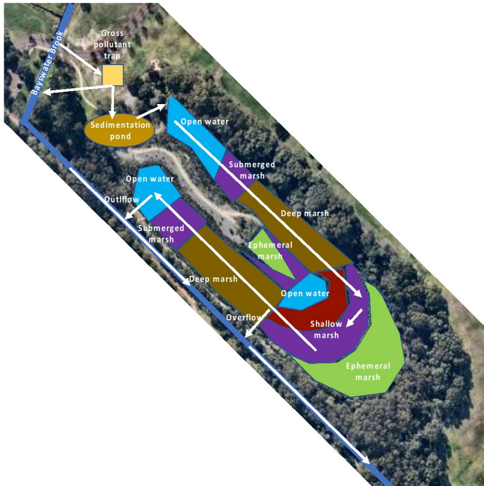
Figure 3 Design components, showing gross pollutant trap, sedimentation pond, open water and different marsh zones, and outflow and overflow to Bayswater Brook (modified from GHD 2013).
