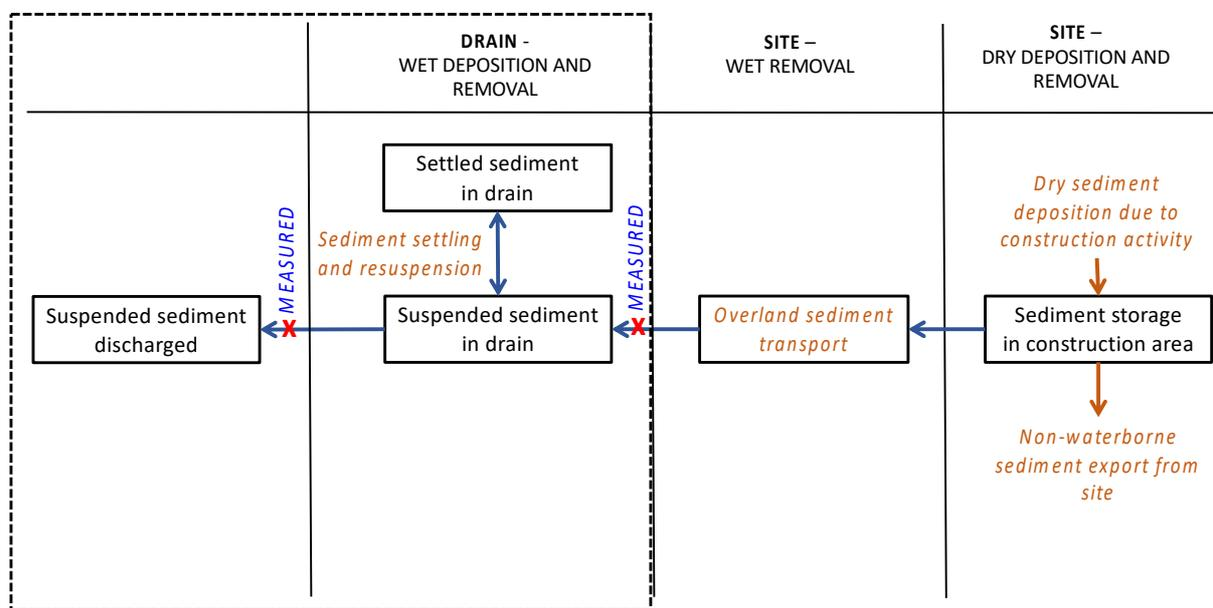
Figure 2 Schematic of soil erosion from land development sites, incorporating air-borne erosion and water-borne erosion. This project focused on quantifying water-borne erosion.
