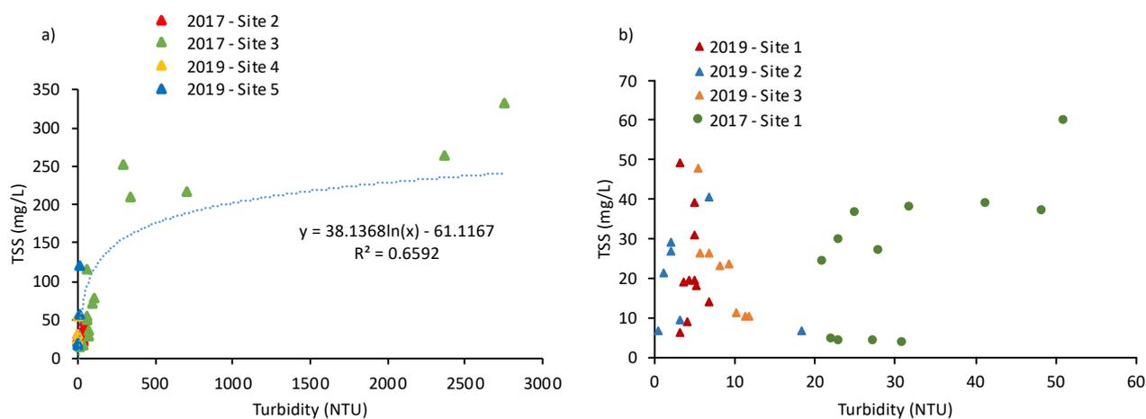
Figure 6 Relationship between total suspended solids (TSS) and turbidity, measured in 2017 and 2019, in a) drains receiving water from areas under construction, and b) drains receiving water from areas no longer under construction. Lots on the latter areas had been fully constructed and landscaped. Note the large differences in scale on both the x- and y-axes.
