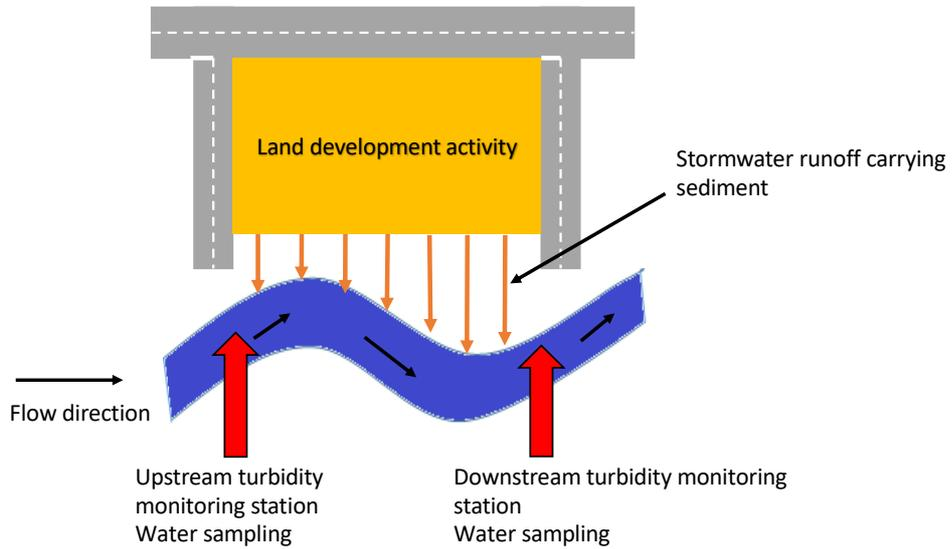
Figure 3 Monitoring approach used for the project; measuring turbidity upstream and downstream of a specific land development activity.
