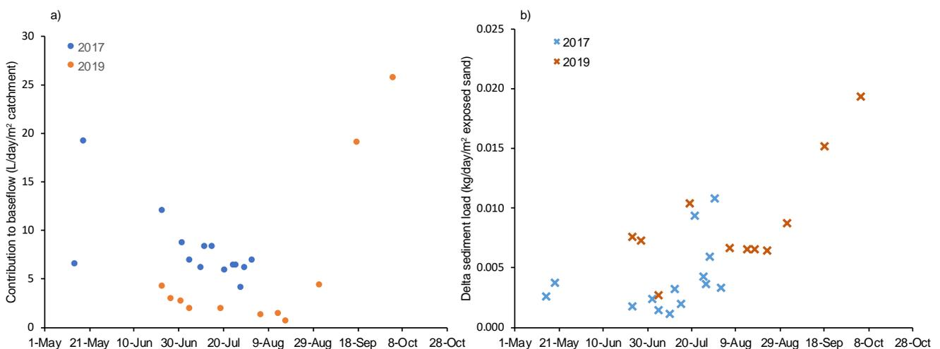
Figure 7 a) Additional flows measured at S2 compared to S1, under baseflow conditions in 2017 and 2019, relative to the Stage 23 sub-catchment area discharging to the drain; and b) change in sediment load per day per square metre of exposed sand, from S1 to S2 over the same monitoring periods in 2017 and 2019.
