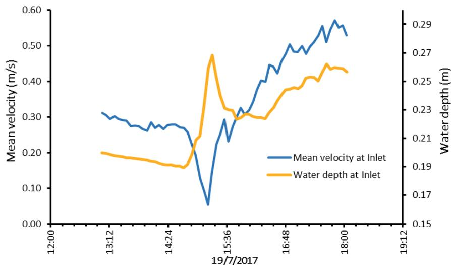
Figure 5 Mean velocity and water depth for event on 19<sup>th</sup> July 2017 at station S1. The decrease in water velocity just after 15:00 corresponded to the establishment of downstream control during peak water levels.
