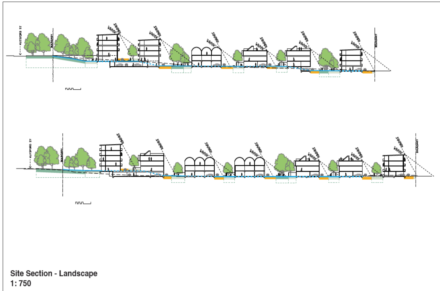
Figure A11: Cross-section of the maximised water sensitive scenario (WS-Max), and including landscape services
