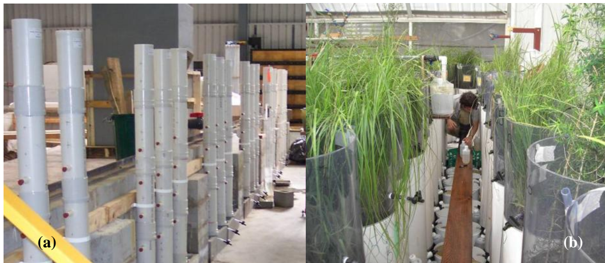
Figure 4. Laboratory biofilter column experiments: (a) non-vegetated soil filter media columns and (b) standard columns
